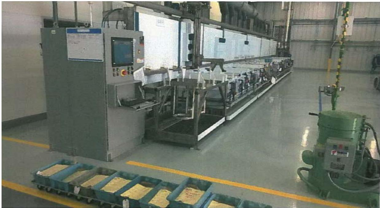
*Figure 1: The newly installed plating line*
