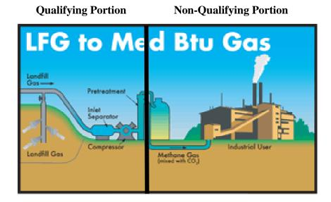
Landfill Gas-to-Medium Btu Gas Processing Project at Montauk
