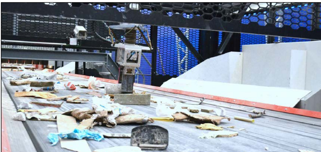
Figure 1: ZenRobotics automated sorting system
